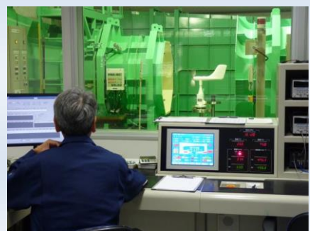
Verification of a Wind Vane/Anemometer
